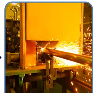
Automatic Pipe Cutting
