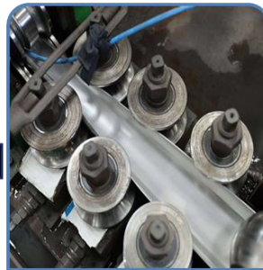
Automatic Pipe Molding
